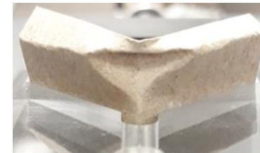
Buckling as failure behavior
